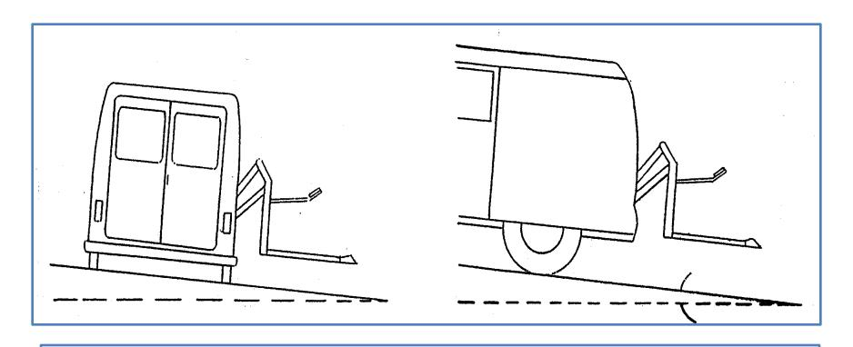
These ramps are incorrectly lowered on inclines. You can see how a wheelchair could roll off of the ramp and down the slopes.
